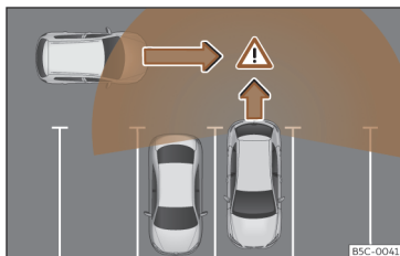
Fig. 167 Schematic representation of the rear cross traffic alert assistant: zone monitored around the vehicle while leaving a parking space.
