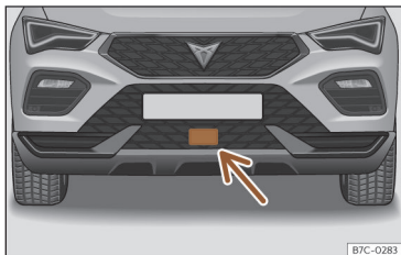
Fig. 143 On the front bumper: radar sensors.
