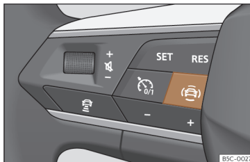
Fig. 58 Left side of the multifunction steering wheel: button for driver assistance systems (depending on versions).
