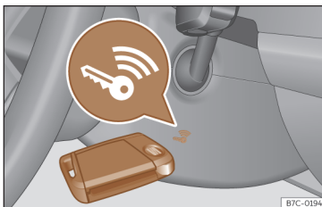
Fig. 135 On the right of the steering column» Fig. 135, as close as possible to the Kessy logo.
