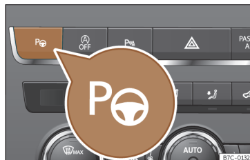
Fig. 170 In the upper part of the centre console: button to switch on the Park Assist system.
