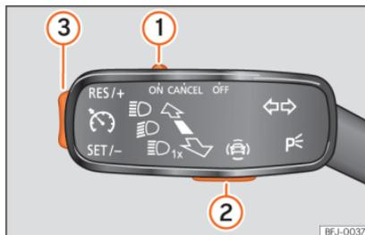
**Fig. 224** On the turn signal lever: buttons to operate the speed limiter.
