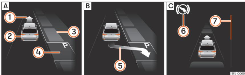
**Fig. 254** On the instrument panel display: parallel parking. **[A]** Finding a parking space. **[B]** Parking position. **[C]** Manoeuvring.
