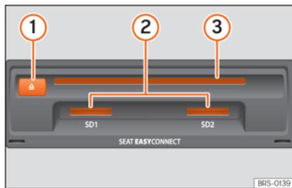
**Fig. 184** Slots for data storage devices in the glove compartment.
