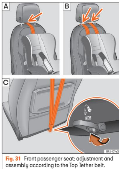
**Fig. 31** Front passenger seat: adjustment and assembly according to the Top Tether belt.
