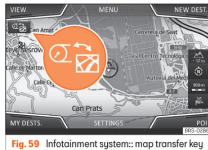
Fig. 59 Infotainment system:: map transfer key
