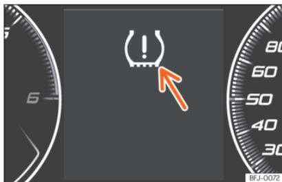
**Fig. 292** Instrument panel: warning of loss of tyre pressure.
