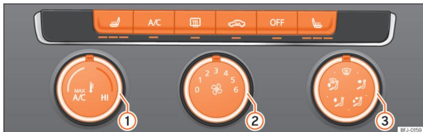
**Fig. 154** In the centre console: manual air conditioning controls.
