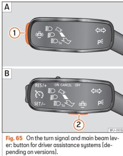
**Fig. 65** On the turn signal and main beam lever: button for driver assistance systems (depending on versions).
