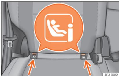
**Fig. 28** Side seats of the second row: ISOFIX/i-Size securing rings.
