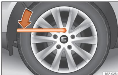
**Fig. 38** Wheel change: loosen the wheel nuts.
