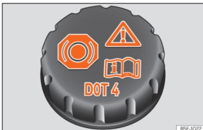
**Fig. 287** Engine compartment: brake fluid reservoir cap.
