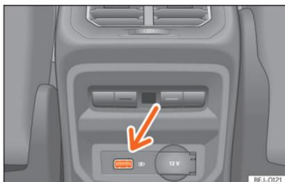
**Fig. 207** Rear part of the centre console: USB connectors.
