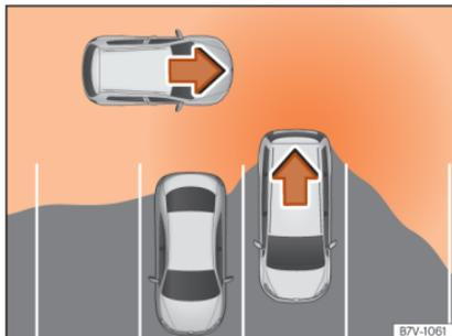
**Fig. 247** Schematic representation of the rear cross traffic alert assistant: zone monitored around the vehicle while leaving a parking space.
