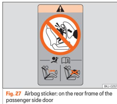
**Fig. 27** Airbag sticker: on the rear frame of the passenger side door
