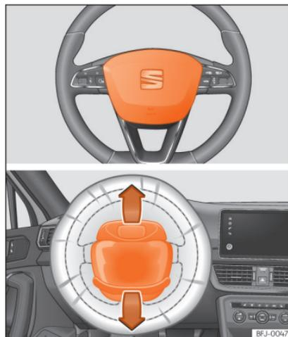
**Fig. 16** Driver airbag located in steering wheel.
