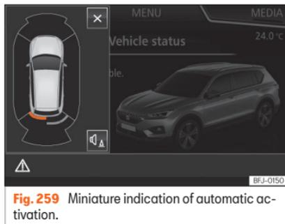
**Fig. 259** Miniature indication of automatic activation.
