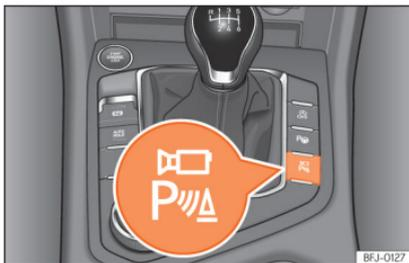
**Fig. 266** Centre console: button to manually activate/deactivate the peripheral vision system when combined with the park assist system.
