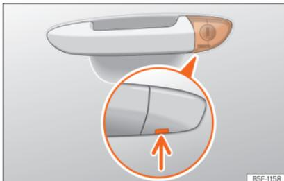
**Fig. 80** Driver door handle: Concealed lock cylinder.
