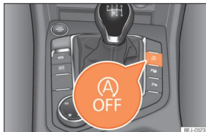
**Fig. 213** Centre console: Start-stop system button.
