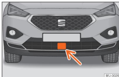
**Fig. 228** On the front bumper: radar sensors.
