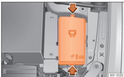
**Fig. 54** In the engine compartment: fuse box cover.
