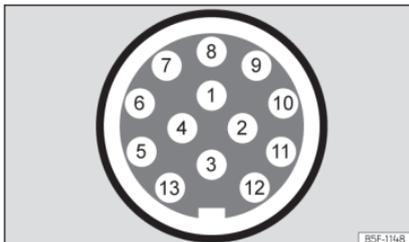
**Fig. 272** Schematic representation: assignment of the pins of the trailer's electrical socket.
