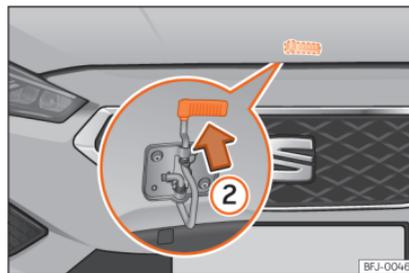
**Fig. 281** Cam under the bonnet
