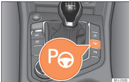
**Fig. 251** In the upper part of the centre console: button to switch on the Park Assist system.
