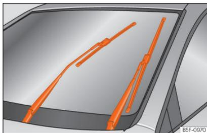
**Fig. 43** Wipers in service position.
