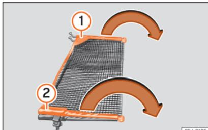
**Fig. 135** Deploying the net partition.
