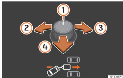
**Fig. 263** Rotary exterior mirror controls.: adjust the trailer angle.
