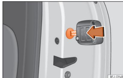
**Fig. 82** Locking the door manually.
