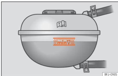
**Fig. 285** In the engine compartment: marking on coolant expansion tank.
