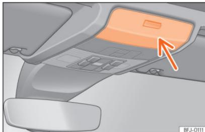
**Fig. 143** On the roof console: glasses case.
