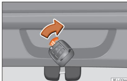
**Fig. 88** Detail of the luggage compartment: emergency unlocking
