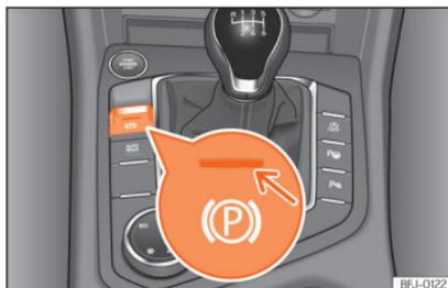
**Fig. 248** In the lower part of the centre console: electronic parking brake button
