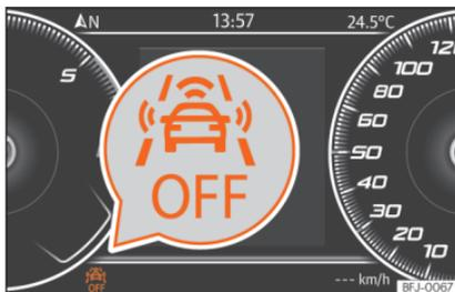
**Fig. 229** On the instrument panel display: Front Assist deactivated indication.
