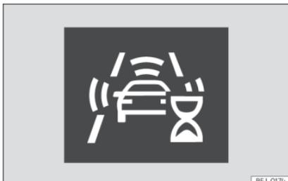
**Fig. 230** On the instrument panel display: initial system self-calibration indication.
