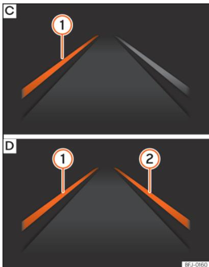
**Fig. 242** On the instrument panel display: Indication on the Lane Assist system display (example 2).
