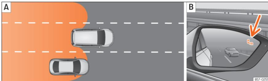
**Fig. 246** Schematic representation: **A** Situation of passing and then moving into the right-hand lane. **B** Indication from the blind spot detector in the right-hand external mirror.
