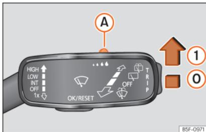
Fig. 102 Wiper lever: adjust the rain sensor **A**
