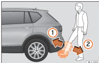
**Fig. 87** Rear lid with sensor-controlled opening [Easy Open].
