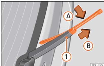
**Fig. 45** Changing the rear wiper blade
