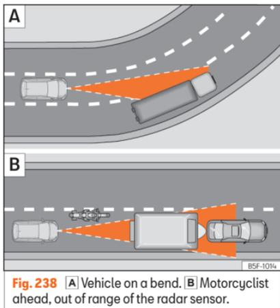
**Fig. 238** [A] Vehicle on a bend. [B] Motorcyclist ahead, out of range of the radar sensor.
