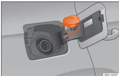
**Fig. 275** Fuel tank flap with tank cap attached.
