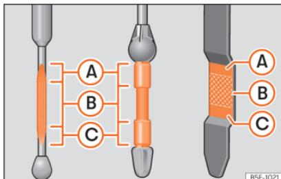
**Fig. 283** Engine oil dipstick.
