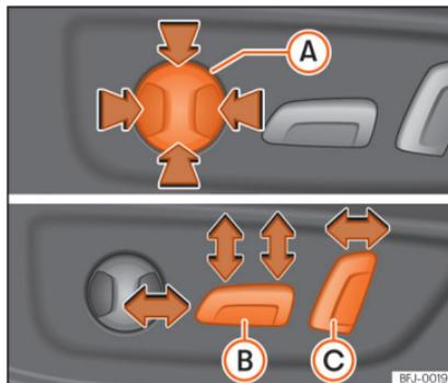
Fig. 108 Driver's seat: electric seat settings.
