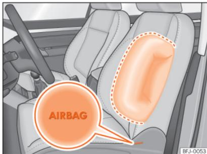
**Fig. 22** Side airbag in driver's seat.
