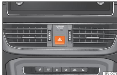
**Fig. 98** Dash panel: hazard warning lights switch
