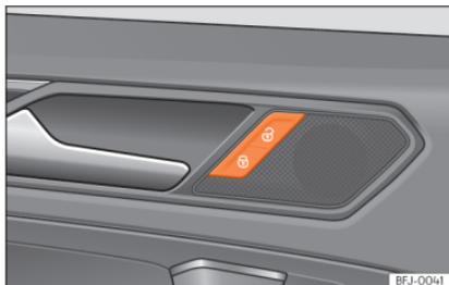
**Fig. 76** Driver's door: central locking switch.
