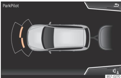
**Fig. 261** Parking assist display on the screen with trailer attached.
