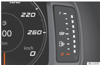
Fig. 62 Digital instrument panel: fuel gauge.
