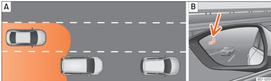
**Fig. 245** Schematic representation: **A** Passing situation with traffic behind the vehicle. **B** Indication from the blind spot detector in the left-hand external mirror.
