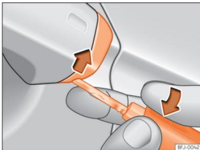
**Fig. 81** Driver door handle: lever the cover off
