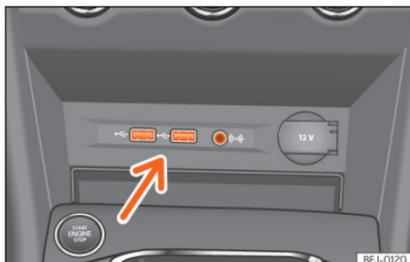
**Fig. 206** Centre console: USB/AUX-IN input.
