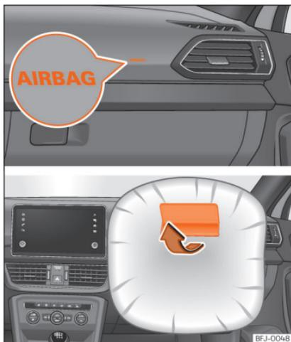
**Fig. 17** Front passenger airbag located in dash panel.
