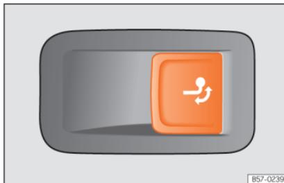
**Fig. 273** On the right side of the luggage compartment: button for unlocking the tow hook.
