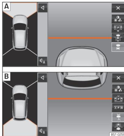
**Fig. 267** Display on the top view system screen: [A] Front camera: off-road view. [B] Rear camera: off-road view.
