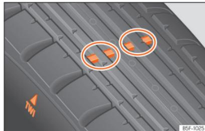
Fig. 290 Tyre profile: tread wear indicators.
