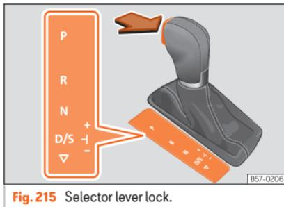
**Fig. 215** Selector lever lock.
