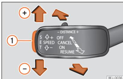
**Fig. 225** On the left of the steering column: buttons to operate the speed limiter.
