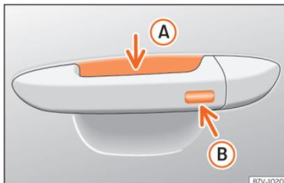
**Fig. 79** Door handle: sensor surfaces
