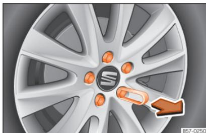
Fig. 36 Wheel: wheel nuts with caps.
