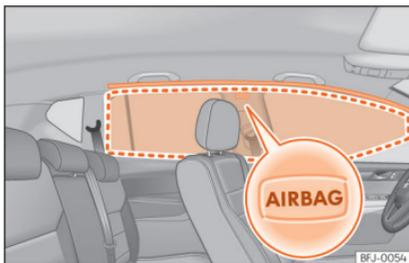
**Fig. 23** Location of head-protection airbags.
