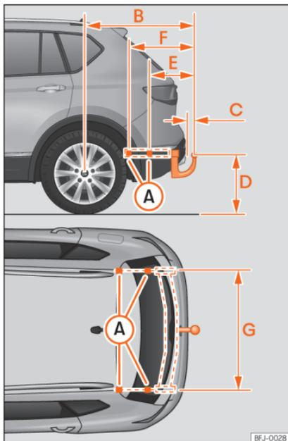
**Fig. 274** Limits and attachment points for retrofitting a towing bracket.
