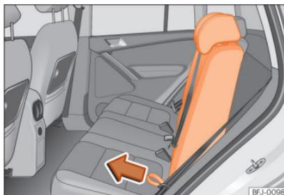
Fig. 119 Folding down and lifting the rear seat backrest
