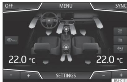
**Fig. 155** Easy Connect screen: Climate control menu.
