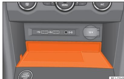
**Fig. 209** In the centre console: pad for the mobile phone connection.
