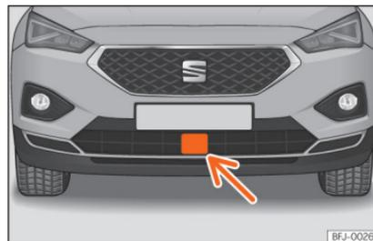
**Fig. 234** On the front bumper: radar sensors.
