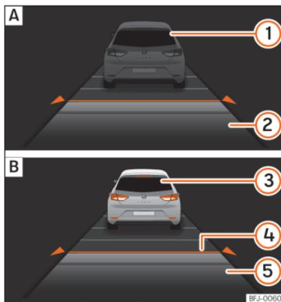
**Fig. 233** On the instrument panel display: [A] ACC inactive (Standby). [B] ACC active.
