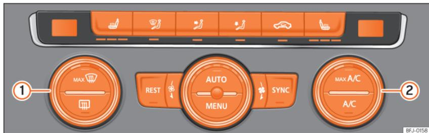
**Fig. 153** In the centre console: Climatronic controls.
