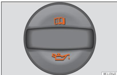
**Fig. 284** In the engine compartment: Engine oil filler cap.
