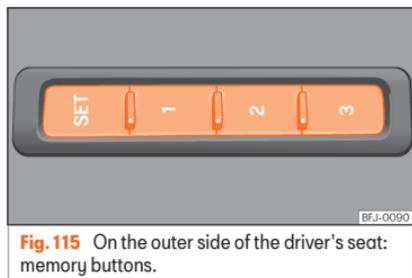
**Fig. 115** On the outer side of the driver's seat: memory buttons.
