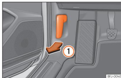
**Fig. 280** Release lever in the driver's footwell area.
