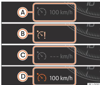
**Fig. 221** Instrument panel display: GRA status indications.
