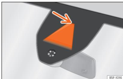
**Fig. 240** On the windscreen: field of vision of the Lane Assist system.
