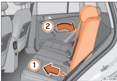
**Fig. 110** Rear seat backrest adjustment.
