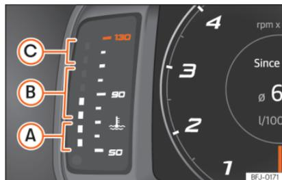
Fig. 63 Digital instrument panel: engine coolant temperature indicator.
