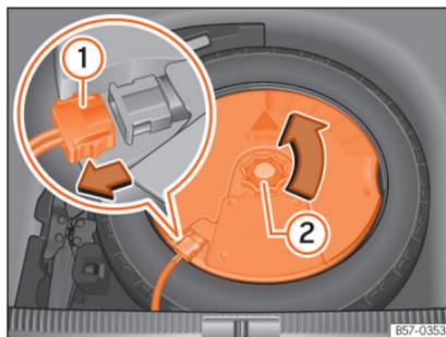
**Fig. 294** In the luggage compartment: remove the subwoofer.
