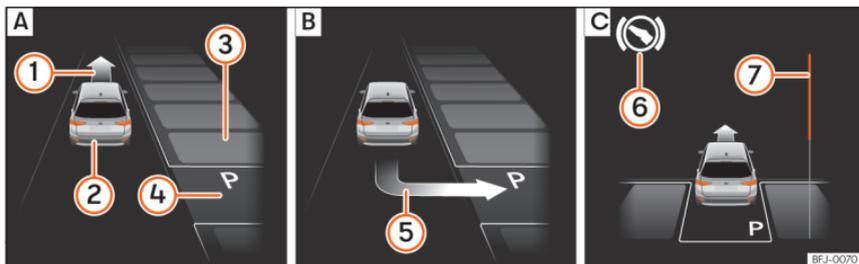
**Fig. 255** On the instrument panel display: angle parking. **[A]** Finding a parking space. **[B]** Parking position. **[C]** Manoeuvring.
