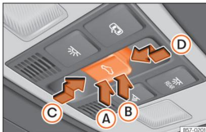
**Fig. 90** On the interior roof lining: sunroof button.
