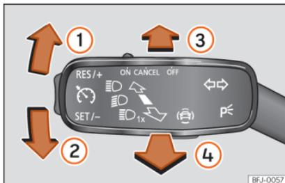
**Fig. 96** Turn signal and main beam lever.
