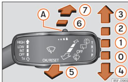
**Fig. 101** Operating the windscreen wiper and rear wiper.
