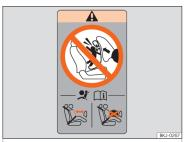
Fig. 27 Airbag sticker: on the rear frame of the passenger side door
