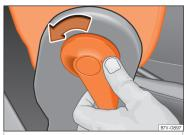
Fig. 118 Unlocking the folding backrest of the front passenger seat
