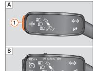
Fig. 65 On the turn signal and main beam lever: button for driver assistance systems (depending on versions).
