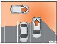
Fig. 247 Schematic representation of the rear cross traffic alert assistant: zone monitored around the vehicle while leaving a parking space.
