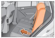
Fig. 119 Folding down and lifting the rear seat backrest
