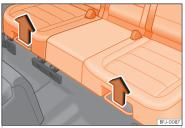
Fig. 109 Under the bench of the rear seat: setting levers.
