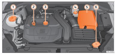
From time to time, the levels of the different fluids in the vehicle must be checked. Never
