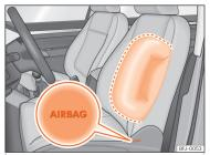
Fig. 22 Side airbag in driver's seat.
