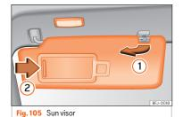
Options for adjusting driver and front passenger sun visors
